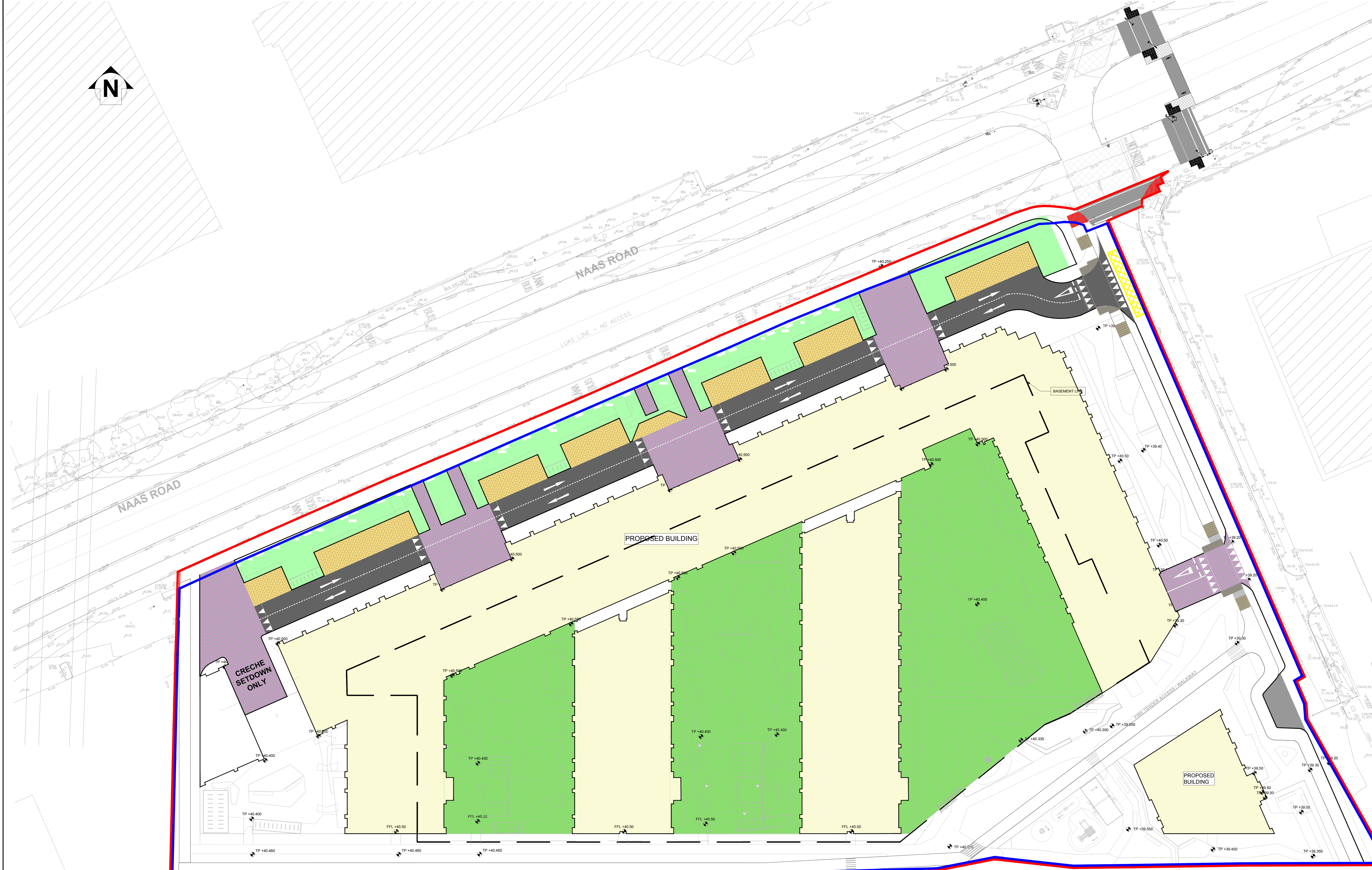
PROPOSED SUDS LAYOUT SCALE @ A0: 1:200 SCALE @ A2: 1:500
